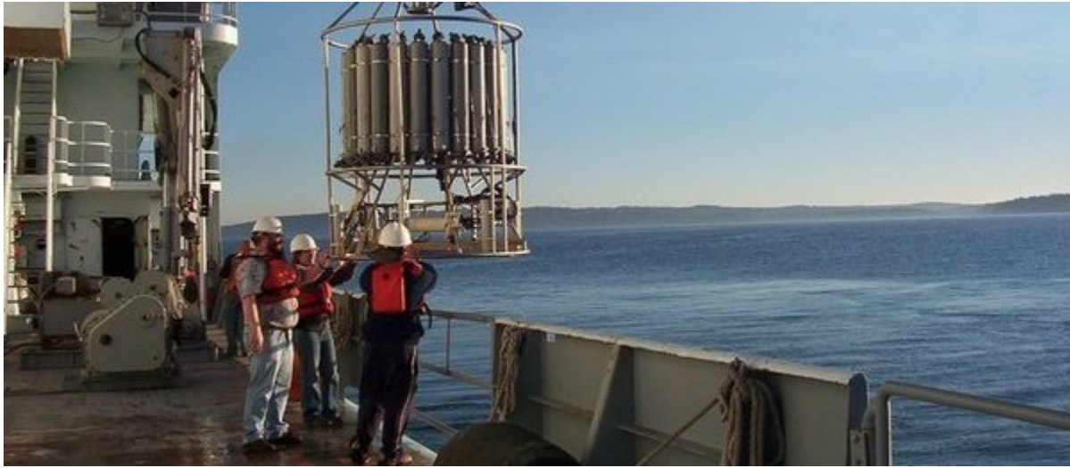
Figure 4. Center research scientist Finn Krogstad and Center graduate student Michele Guannel work with research technician Eric Coker to guide a rosette of water sampling bottles and an instrument to measure salinity and temperature overboard as part of the Center's 2006 interdisciplinary research cruise exploring links between Oceans and Human Health. Photo by Alison Scherer.
